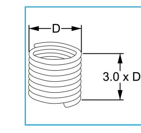
D Pack Packaging dimensions Gross weight EAN Code M 14 x 1.0 mm 10 125x110x40 h mm 0,01 kg 8012667367299
